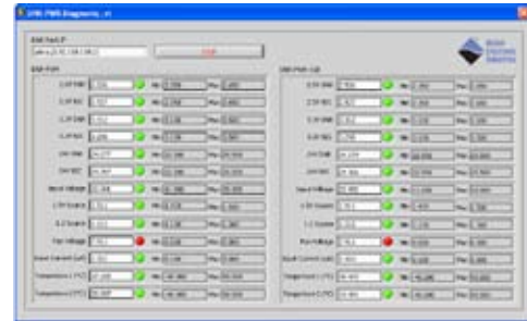
The powerful diagnostics software shown above monitors all system power supplies, temperatures and fan operation.
