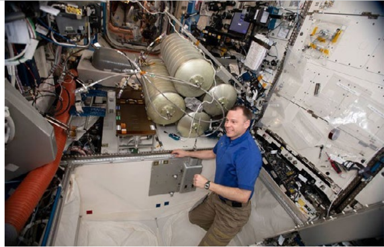
(May 29, 2019) NASA astronaut Nick Hague assembles and installs the Water Storage System inside the U.S. Destiny laboratory module.
