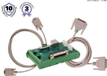
The DNR-BRICK-4-DIAG kit provides easy connections to the 25-pin D-Sub diagnostic/power/sync connector. Power (for non POE or backup) connections are provided via standard UEI power supply Molex connectors. RS-232 connections are through a 9-pin D-Sub connector while sync connections are through an RJ-50 connector. The kit contains:
