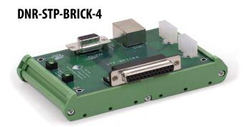
The optional DNR-STP-BRICK-4 (shown at left) provides easy connections to the 25-pin D-Sub diagnostic/power/sync connector. Power (for non POE or backup) connections are provided via standard UEI power supply Molex connectors. RS-232 connections are through a 9-pin D-Sub connecto'r, while sync connections are provided via a RJ-50 connector. Please see the accessories section below for order info.
