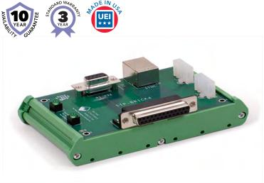
The DNR-STP-BRICK-4 provides easy connections to the 25-pin D-Sub diagnostic/power/sync connector. Power (for non POE or backup) connections are provided via standard UEI power supply Molex connectors. RS-232 connections are through a 9-pin D-Sub connector while sync connections are through an RJ-50 connector. The following cables provide connection to the DNR-BRICK-4 chassis:
