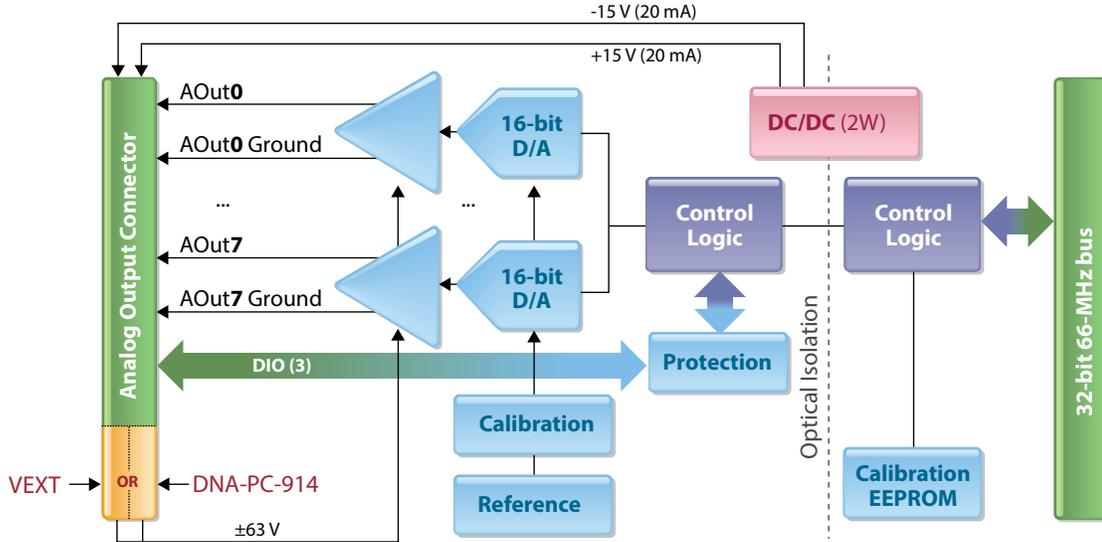
**Figure 1-1. Block Diagram of the AO-308-354 Layer**
