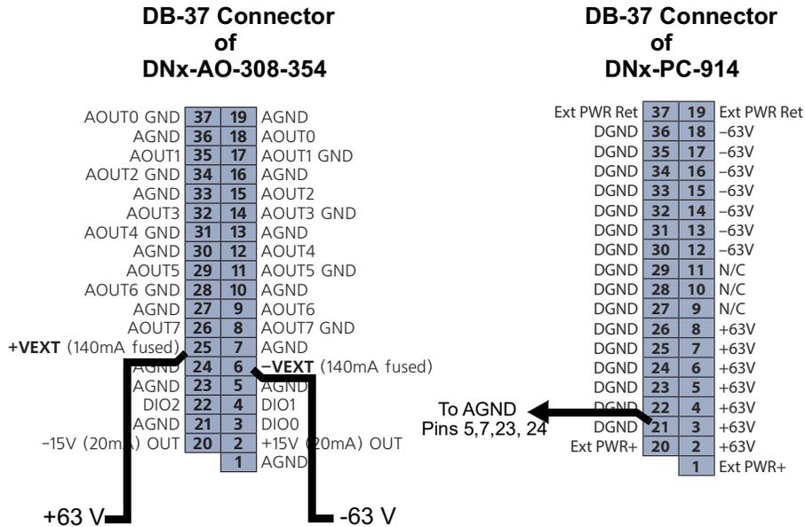
Connect -63 V external power to Pin 6 of DNx-308-354 DB-37 connector.
