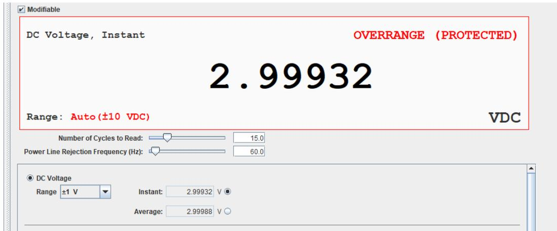
**Figure 3-3 Protection Tripped Indicator**
