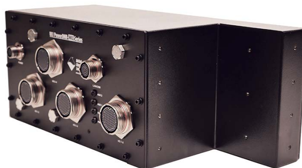
The UEI-HUMS1 provides 8 I/O slots and uses standard DNR-series I/O boards (e.g. DNR-AI-255).
