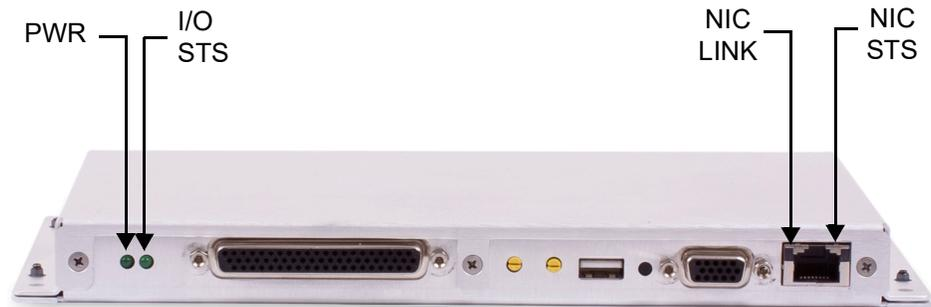
**Figure 2-29 UEI-PIO-1010 (in Optional Case) Status LEDs**
