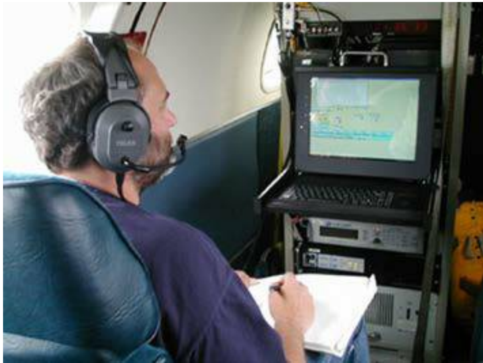
Fig 1 – A small rack holds all the equipment in the airborne LIDAR, a QNX-based system that digitizes inputs from a telescope to help researchers locate various fish species during an efficient air survey. When the operator sees something of specific interest on the display, he can push a button to insert a marker into the datafile to make it easier to find that point during post-acquisition analysis.
