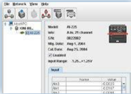
Figure: Floating values read when testing reading on the AI-225.
