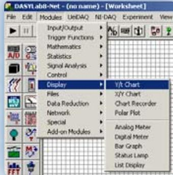
When the Y/t Chart block is created, simply connect the output of the Analog Input Block to the input of the Y/t chart in order to display data that will be acquired in this chart:
