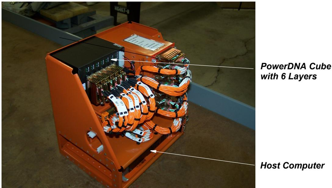
**Figure 2. Cessna Micro-Pak In-Flight DAQ System**
