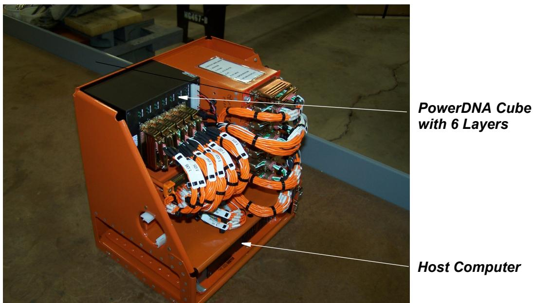
**Figure 2. Cessna Micro-Pak In-Flight DAQ System**
