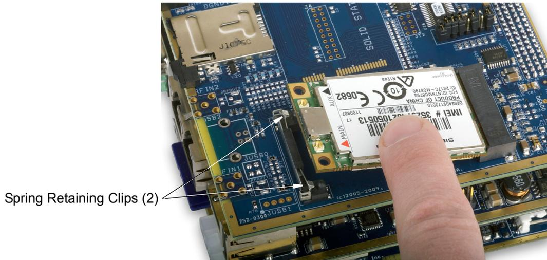
**Figure 1-5. Inserting/Removing PCI Express Mini Wireless Card**
