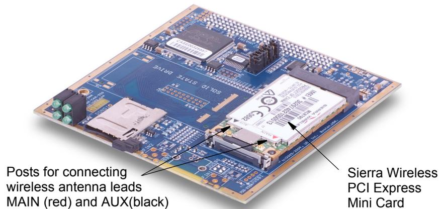
**Figure 1-1. DNA-CAR-550 PCI Express Mini Card Module Carrier Board**
