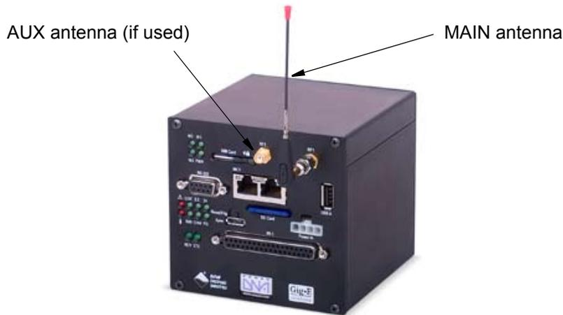
**Figure 1-2. UEIPAC Cube with CAR-550 Module Carrier**
