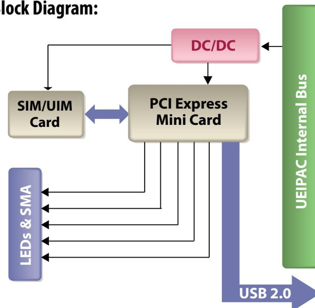
**Figure 1-4. Block Diagram of DNA-CAR-550**
