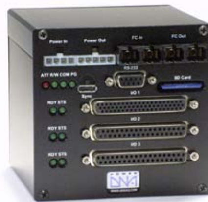
Core Module consists of NIC and PowerPC CPU layers stacked on top of each other and packaged in light-weight aluminum chassis.
