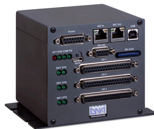
Core Module consists of NIC and PowerPC CPU layers stacked on top of each other and packaged in light-weight aluminum chassis.
