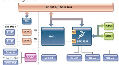
The Core module also provides provides the 8347 series PowerPC CPU, two USB 2.0 controller ports, indicator lights, timing/trigger interface, configuration ports and internal power supply. It's the brains of the Cube and controls the unit's operations including the interface with the host Controller (and other Cubes) and supervising the activity of the I/O Layers.
