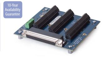
The DNA-STP-62-ES1 provides easy screw terminal connections for all DNx series I/O boards which utilize the 62-pin connector scheme. The DNA-STP-62-ES1 is connected to the I/O board via either DNA-CBL-62 series cables.
