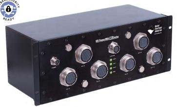
The DNR-MIL provides 12 I/O slots and uses standard DNR-series I/O boards (e.g. DNR-AI-217). It is available in the standard PowerDNR configuration or as a UEIPAC or UEISIM.
