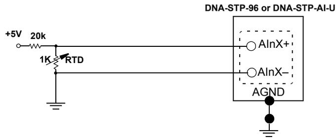
**Figure 1-5. Analog Input Configuration — RTD and Bridge Wiring**
