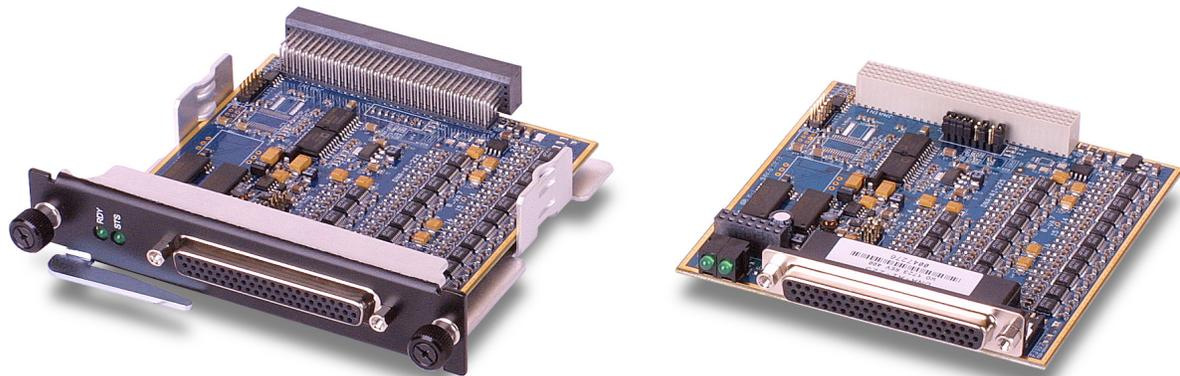
**Figure 1-2. Photos of DNR- and DNA-AI-225 Analog Input Layer Boards**
