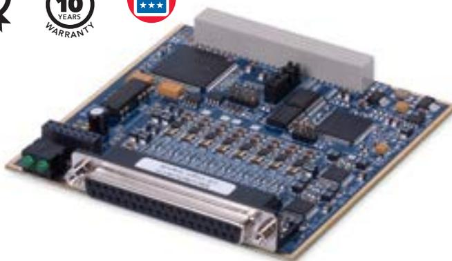
DNA-AO-308-354 shown. When ordered with DNA-PC-914 power conversion board, the DNA-AO-308-354 is factory-configured for internal power. The DNR/DNF-AO-308-354 requires the power supply to be connected externally.
