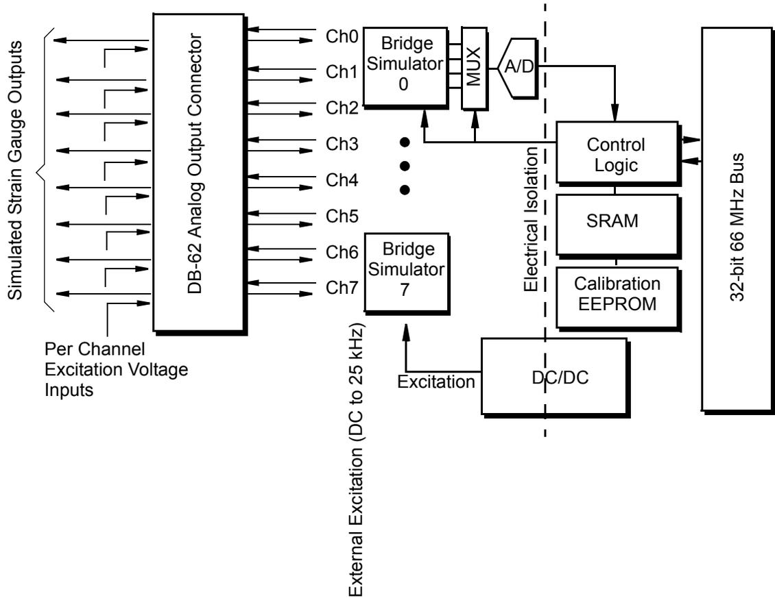
Figure 1-1. Block Diagram of the AO-358 Layer
