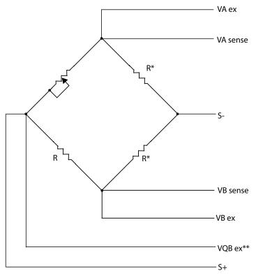
\* Not installed on -QH version of boards
