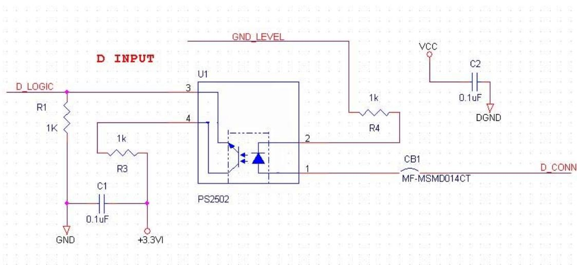
To switch input to a logical one, the user should provide current flowing through the LED in the optical isolator. The minimum current requirement is 2.4mA. The current is limited by resistor R4 and can be as high as 36mA at the maximum input voltage.
