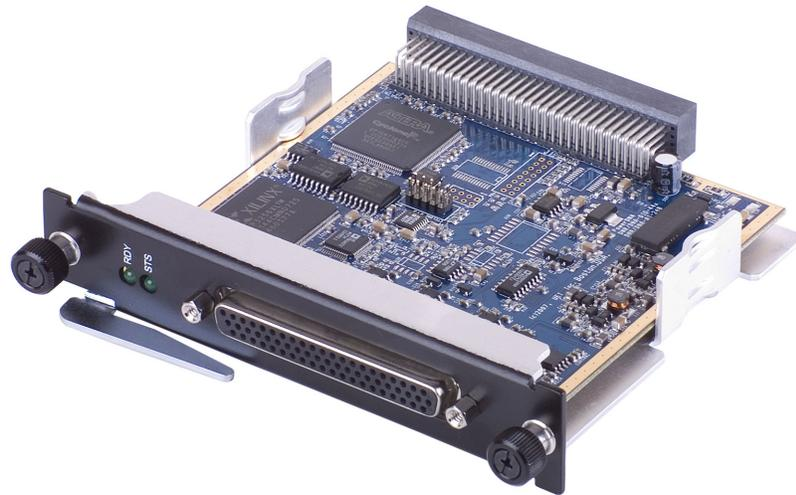
**Figure 1-2. DNR-DIO-448 Digital I/O Layer**
