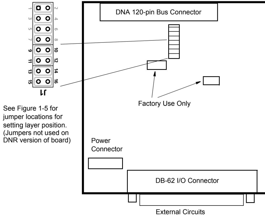
**Figure 1-5. Physical Layout of DNA-DIO-448 Layer Board**
