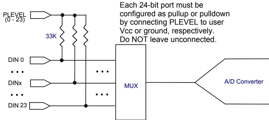
**Figure 1-7. Typical Input Circuit Diagram for Channels 0 to 23 (Port 1)**
