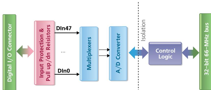
**Figure 1-3 Block Diagram of DIO-448 Device Architecture**
