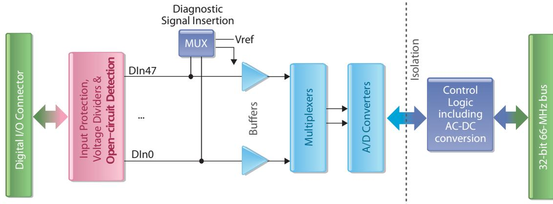
**Figure 1-2. Architecture Block Diagram of DIO-449**
