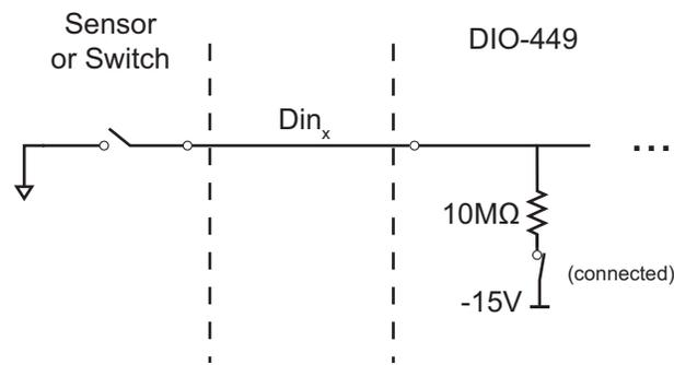
**Figure B-1. GND Open Contact Monitoring with DIO-449**
