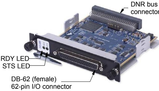
**Figure 1-1. Photo of DIO-449 Digital Input Board**
