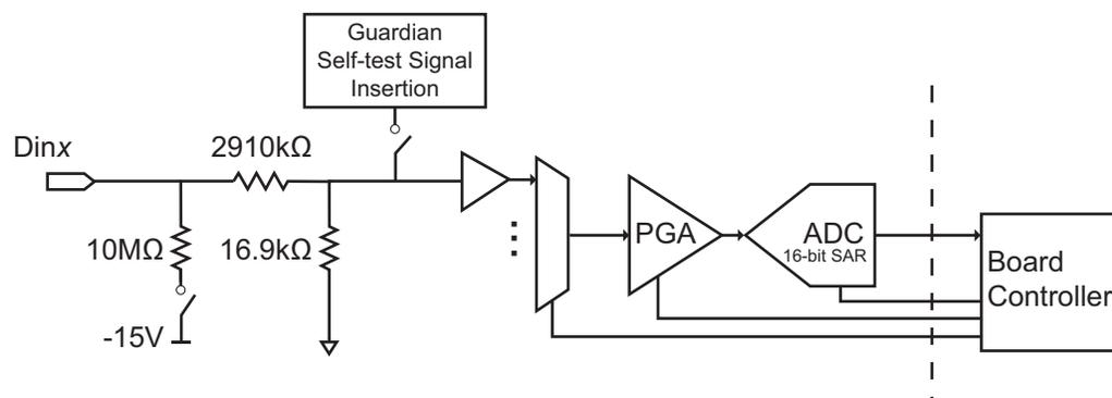
**Figure 1-3. Abstracted Single Channel Diagram for DIO-449**
