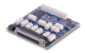
DNA-DIO-462 boards are for use in "Cube" chassis while the DNR-DIO-462 is designed for use in RACKtangle™ chassis, and the DNF-DIO-462 is used in the FLATRACK chassis.
