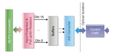
**Notes:** Dout and DIn share the same pin on the I/O connector. Vcc is provided in blocks of 4 channels. To provide proper output functionality with Vcc left open, a 2 M $\Omega$  resistor is connected to an internal 60 V power supply. With neither pull-up/down resistors enabled and the output off, a DMM measurement of the Vcc pin will read approximately +60V. This will not impact functionality with pull-up/down resistors.
