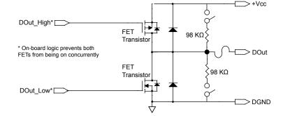
**Notes:** Dout and DIn share the same pin on the I/O connector. Vcc is provided in blocks of 4 channels. DIO-0 through DIO-3 share a Vcc connection as do DIO-4 to DIO-7, DIO-8 to DIO-11 and DIO 12- DIO-15. To provide functionality with Vcc left open, a 2 M $\Omega$  resistor is connected to an internal 60 V power supply.
