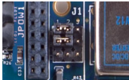
Figure A-4 Photo of PC-91x V+ Power and Ground Connected to Bus 1
