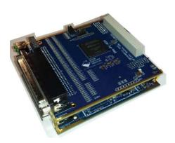
The MAX 10 CPLD daughter-board can be programmed with a custom FPGA design. The FPGA of the base-board interfaces the Altera MAX 10 to the PowerDNA system.
