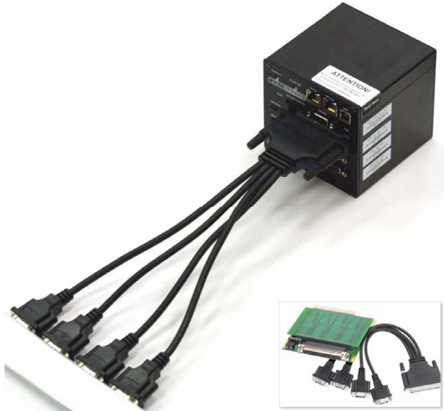
Figure 1-5. PowerDNA Cube with DNA-SL-501 and Cables
