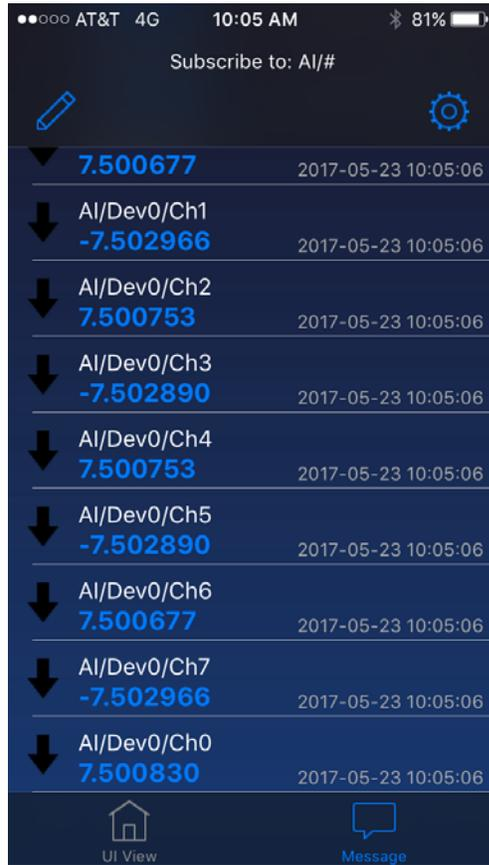
Figure 18: Hand-held Display of Analog Input Data
