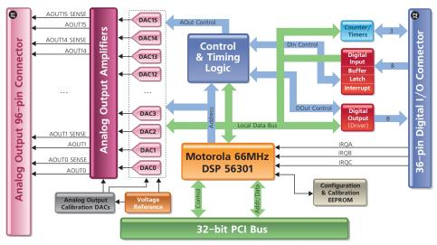
Note: AOUTX on PD2-AO-16/16 board is internally connected to the corresponding AOUTX SENSE line. If you need remote sensing option, please use PD2-AO-32/16HC board.
