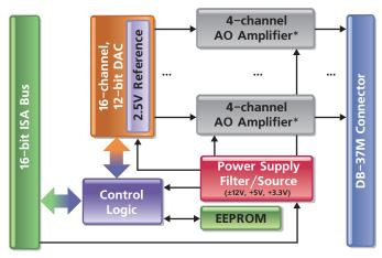
\* Includes range selectors (±2.5V; ±5V; ±10V; 0-5V; 0-10V; 4-20mA) and manual gain/offset calibration circuitry.
