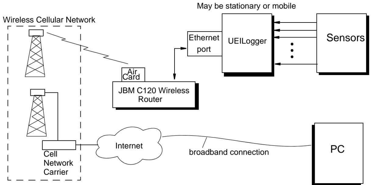
**Figure 1-2. Cellular Wireless UEILogger System (Single or Multi-Cube)**
