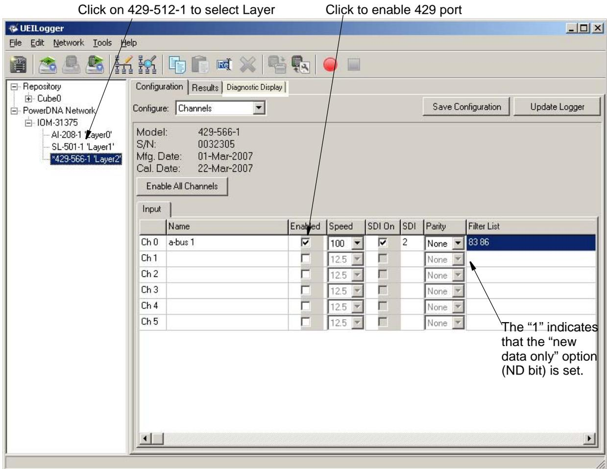
**Figure 2-51**Configuring the 429-512 Ports
