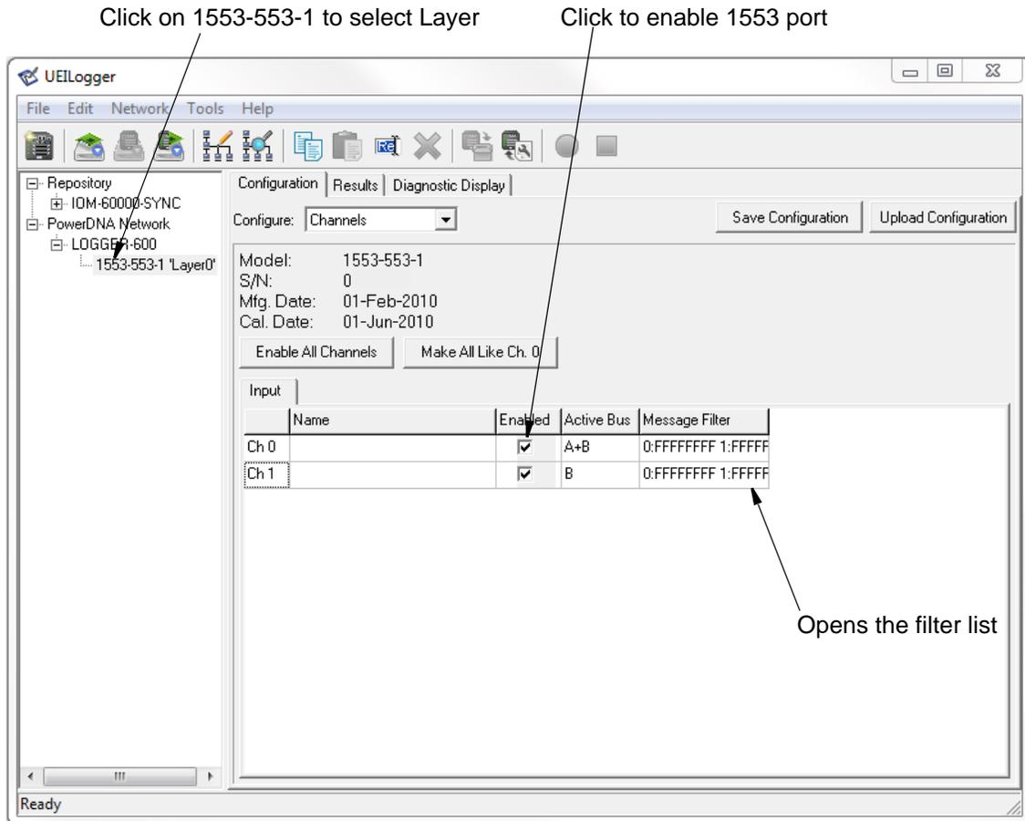
**Figure 2-54** Configuring the 1553 ports
