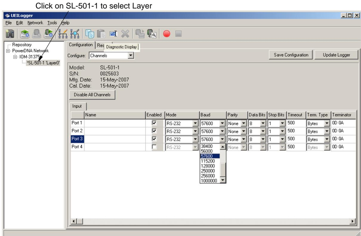
**Figure 2-35** Configuring the SL-501 Ports
