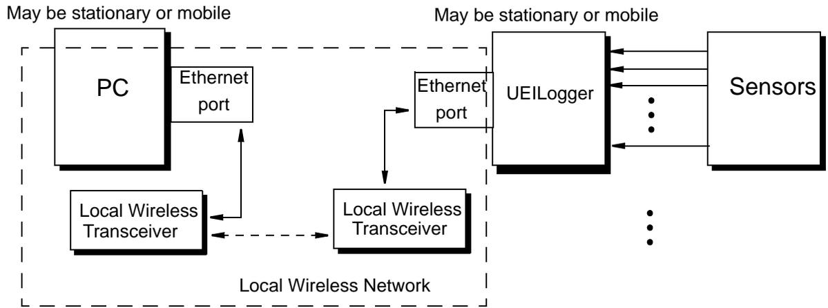
**Figure 1-3. Local Wireless UEI Logger System (Single or Multi-Cube)**
